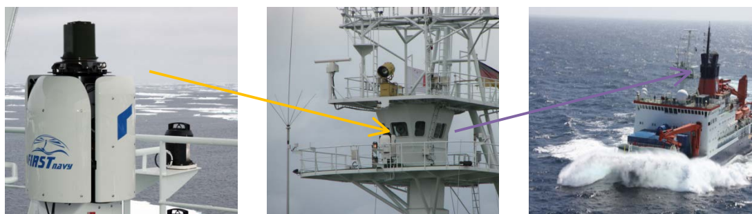
Figure 2. Installation of the AIMMMS Infrared System on RV Polarstern
